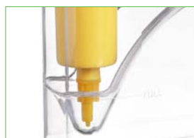
The lower suction head is sealed with the silicone gasket to the bottom of the suction hole to ensure that the saliva is completely sucked into the DNA sample preservation tube.
