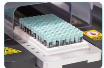
Drawer-style input and output ports to minimize the risk of sample contamination during the lid-opening process.
