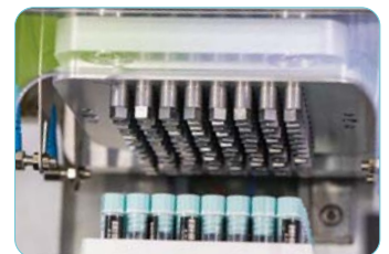
SBS standard cryovials, with quick, safe, and efficient cap operation for the entire box.
