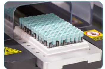
Drawer-style input and output ports to minimize the risk of sample contamination during the lid-opening process.
